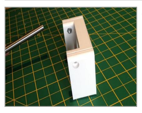
Use two M3 8mm bolts and nuts to clamp the smooth rods into the idler end. The threaded rod should slide through the 625ZZ bearings.
