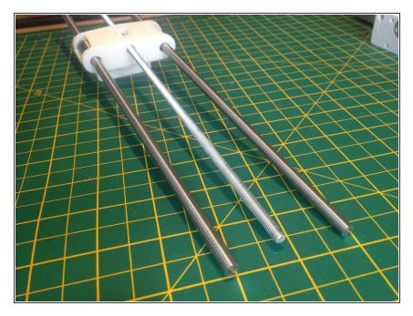
Slide the two smooth rods through the LM6UU linear bearings.
