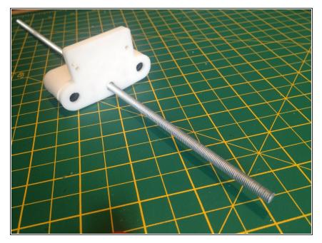
Insert and screw the threaded rod through the trapped M5 nut.
