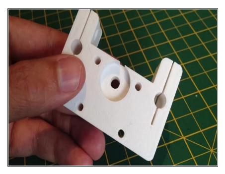
Insert the two 625ZZ bearings into the idler end.
