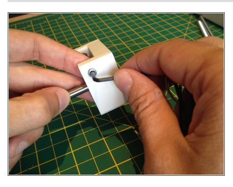
Use two M3 8mm bolts and nuts to clamp the smooth rods into the motor end.
