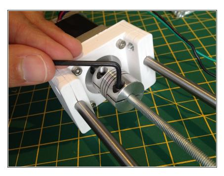
Attach the flexible coupling to the stepper motor and the threaded rod.
