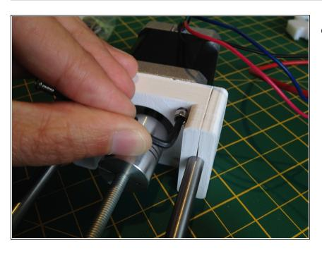
Use four M3 16mm screws to attach the stepper motor to the motor end.
