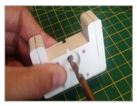
Clean the 3D printed holes using 3mm, 5mm and 6mm drill bits.
