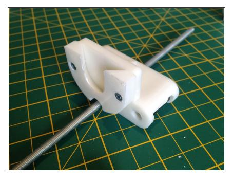
Use two M3 10mm bolts and nuts to attach the syringe plunger retainer to the syringe carriage.
